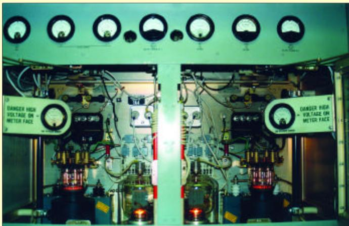
**Figure 9.** A view of two of the 12 PA tubes with filaments lighted. The red hoses carry deionized water around the tube for cooling. Additionally, all the tubes inside the transmitter are cooled by circulating air at 55° F. Photo courtesy of ETI K. McKinley.
