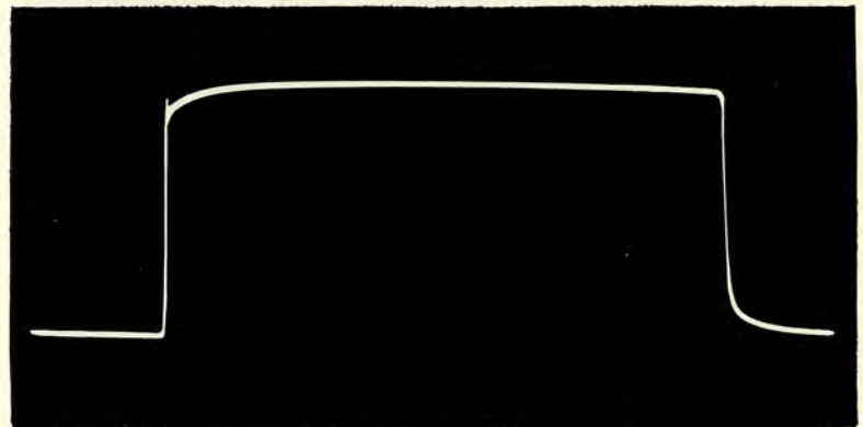
Figure 7-155. Synchronization Indicator, Pedestal Follower Cathode Waveform
