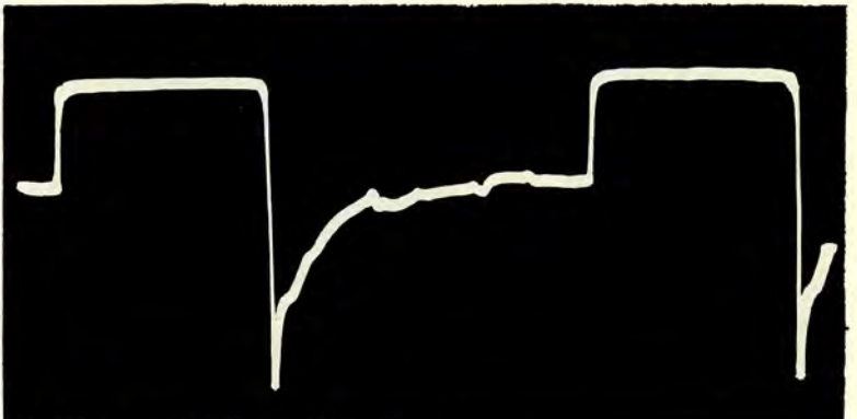
Figure 7-44. Frequency Divider, Counter 1, 4 Stage Output Waveform
