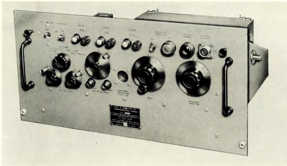
Figure 1-6. Synchronization Control Type C-1238/FPN-30, Front Oblique View
