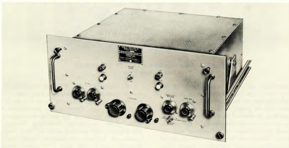
Figure 1-9. Radio Receiver Type R-564/FPN-30, Front Oblique View
