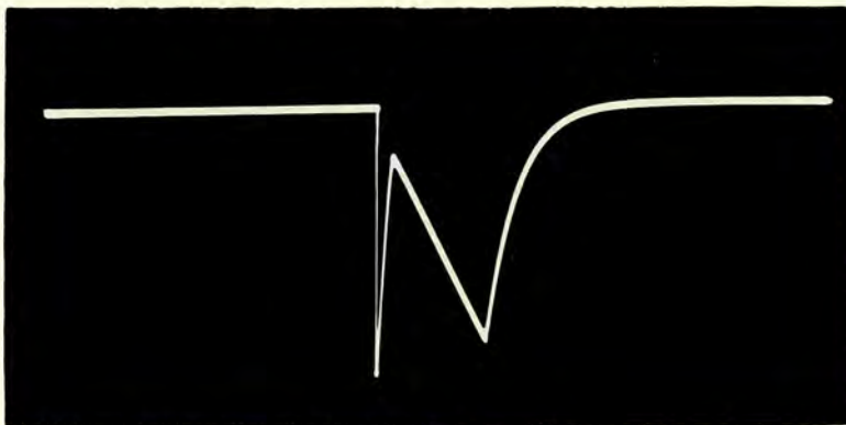
Figure 7-225. Test Scope, Continuous Delay Phantastron Plate Waveform
